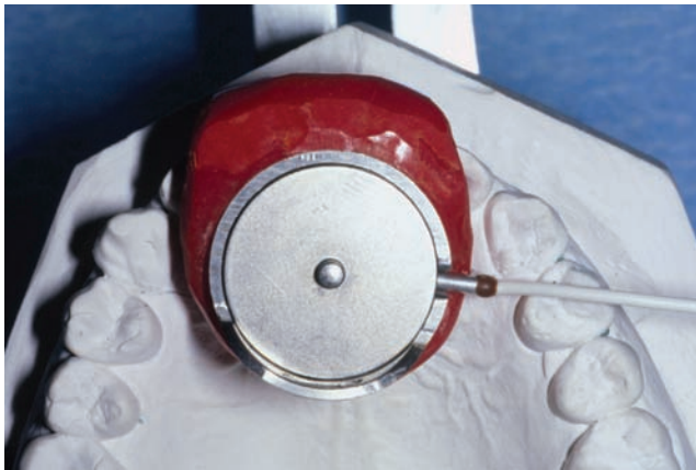
Fig 1. Bite force transducer with stainless steel housing and anterior Duralay resin jig.
